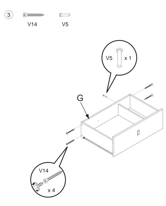
3. Attach back panel (G) to the drawer with screws (V14, V5).
